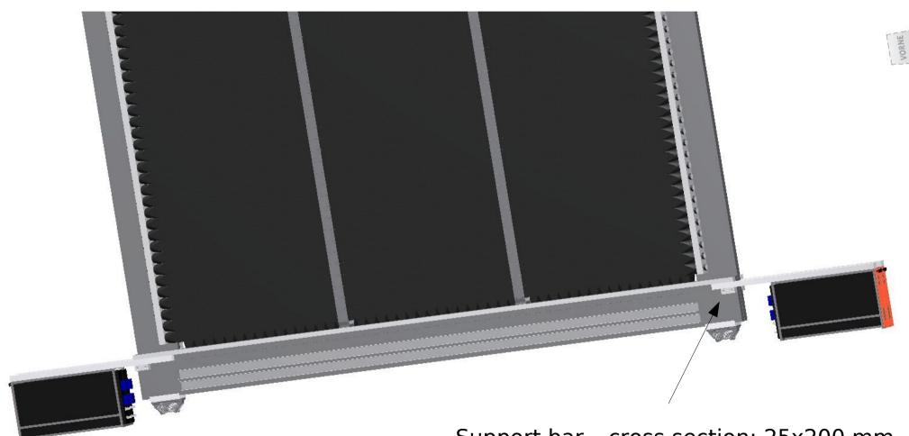
Support bar – cross section: 25x200 mm
