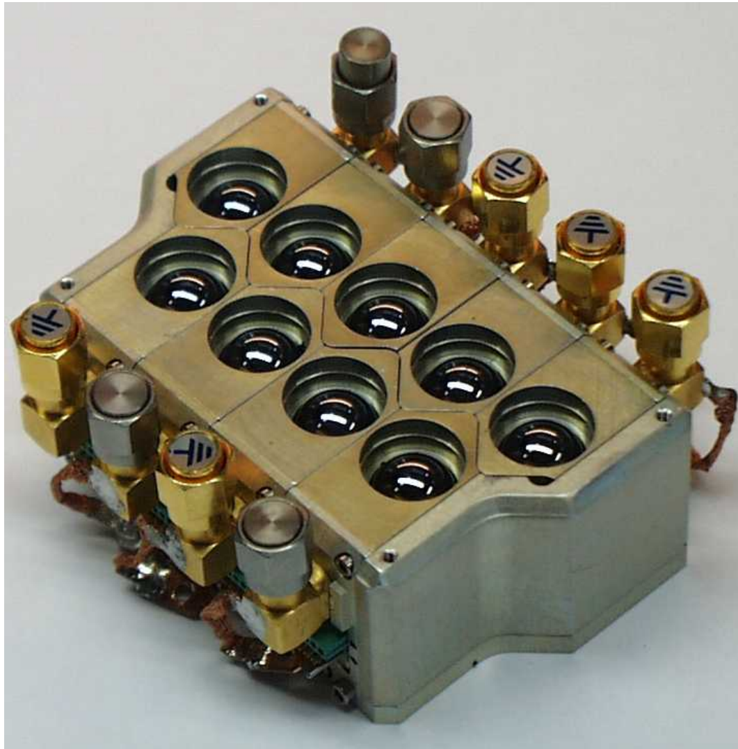
Fig 7. Nine-pixel imaging array receiver block. Each pixel is an independent integrated receiver with its own internal local oscillator. The array mount is shown from the side of its input microwave lenses.
