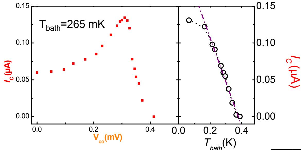
Measurement of the electronic temperature  $T$
