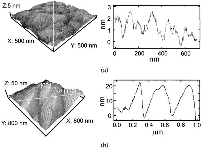
Fig. 2. AFM images of (a) *c*-axis and (b) (110)-oriented YBCO film surfaces (left parts) and the cross-sections (right parts) performed along the white lines on the corresponding left parts. The film thickness is 150 nm in both cases.
