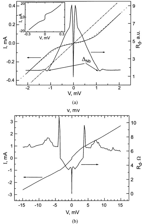
Fig. 3. (a) Typical  $I$ - $V$  and  $R_d(V)$  curves of the Nb/Au/YBCO *c*-HJ with a 20 nm thick Au film, measured at  $T = 4.2 \text{ K}$  (solid lines). The fitting of the  $I$ - $V$  curve to the (1) (dotted line) and the Ohm's law  $V = IR_N$  (dash-dot line) are also shown. The inset presents the  $I$ - $V$  curve at small voltages,  $V \leq 300 \mu\text{V}$ ; (b)  $I$ - $V$  and  $R_d(V)$  curves of the Nb/Au/YBCO *t*-HJ at  $T = 4.2 \text{ K}$ .
