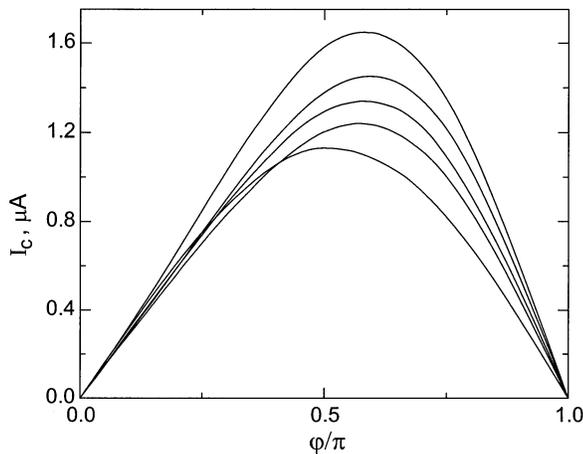
Fig. 5. The experimental current-phase relation of the Nb/Au/YBCO  $c$ -HJ J9 at  $T = 1.7, 2.5, 3.5, 4.2,$  and  $6.0$  K (from top to bottom) measured by the RF-SQUID technique.
