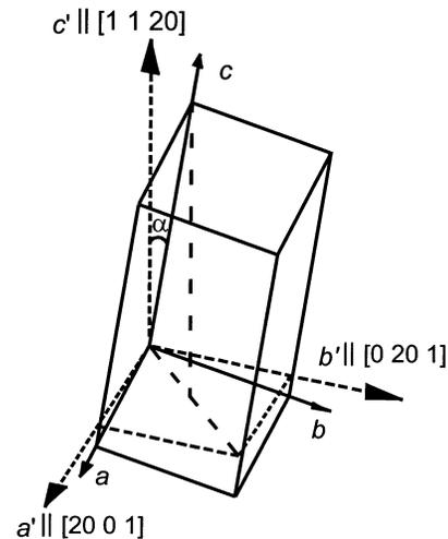
Fig. 1. Schematic of the (1 1 20)YBCO film growth on (7 10 2)  $\text{NdGaO}_3$  substrates. The angles between crystallographic axes *a*, *b*, *c* of (1 1 20)YBCO film and *a'*, *b'*, *c'* of the “standard” (001)-oriented one on (110)  $\text{NdGaO}_3$  substrate are  $aa' = 7.6^\circ$ ,  $bb' = 7.9^\circ$ ,  $\alpha \equiv cc' = 11^\circ$  correspondingly.
