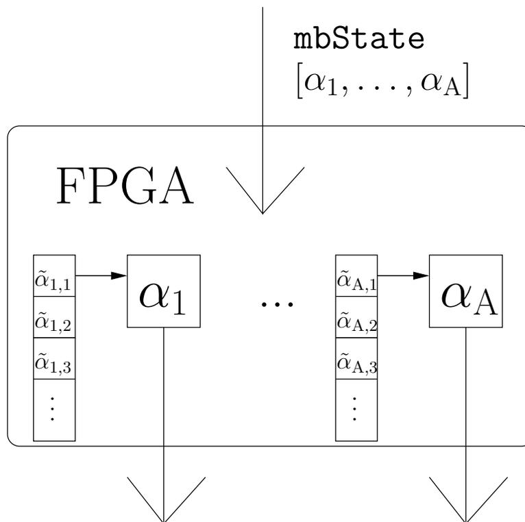
**Figure 6.3:** Structure of the kernels used to identify non-zero matrix elements of one-body operators. The many-body state, consisting of single particle states  $\alpha_i$ , is sent as input. For each single-particle state, one block of hardware is assigned which performs the interchanges of the single-particle state  $\alpha_i$  to a set of new states  $\tilde{\alpha}_{i,j}$ . These processes generate connections in parallel, with individual output-streams to the CPU.
