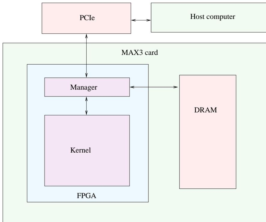
**Figure 5.2:** Schematic view of the MAX3 card and how the different parts are connected to each other. Only parts linked with arrows can directly communicate with each other.
