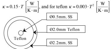
a) Calculate the power with which the coax heats the mixing chamber.
