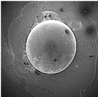
Illustration with the Inlens detector. Although the image shows a very flat illumination of the sample, structures can be recognized which could not be seen on the SE2 image. Material contrast and topography are weak..
