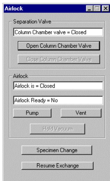
Normally the vacuum will deteriorate due to the locking. Even after closing the separation valve between sample chamber and airlock, the turbo pump will need a certain time to pump the area of the sample chamber to a corresponding vacuum. Opening the V3 valve will only be possible after reaching this limit.
