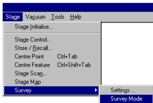
The menu “**Stage**” contains all submenus necessary for control of the motorized stage. Depending on the kind of stage and the number of installed licences, control of the stage is possible in different ways to solve user specific problems or to simplify the work.
