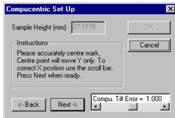
If you want to use the compucentric software also for higher tilt angles, it is recommended to perform the calibration for the next higher tilt angles, too. The stage is to be tilted to  $8^\circ$  now. An eventual drift from the vertical line can be corrected by means of the scroll bar **Compu. Tilt Error**. Clicking the key “Next” will continue the calibration for the following tilt angles in the same way as explained above.
