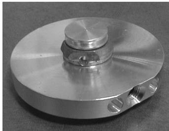
For the calibration a *single sample holder* should be used. It is recommended to use a calibration grid or a TEM grid sample.
