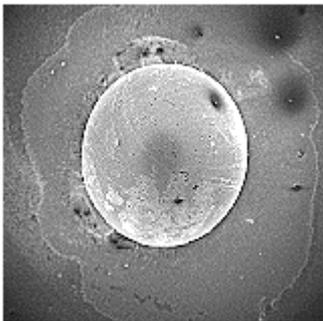
The mixed image between Chamber SE Detector and Inlens SE Detector shows topography and fine structures. The effect can be continuously adjusted.
