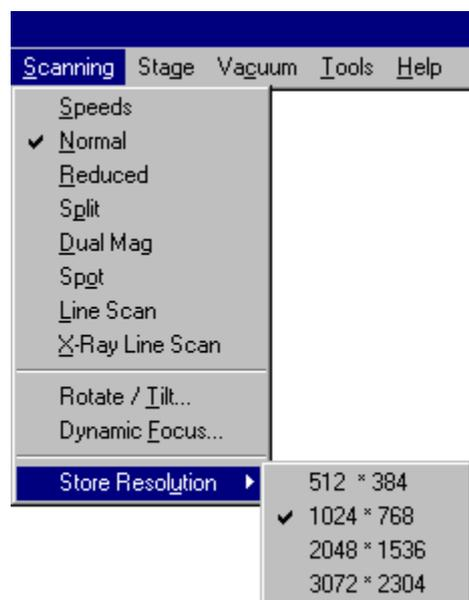
The menu “**Scanning**” contains all necessary options for scanning the sample. Clicking **Speeds** will open a menu for the selection of the different scanning rates. If the license SCANEXP is installed, 15 different scan rates can be selected.
