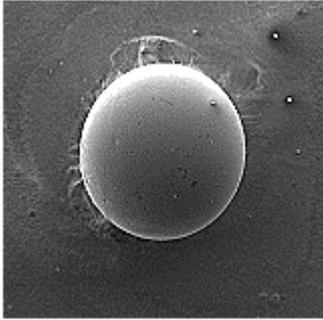
Illustration with the SE2 detector at a positive collector voltage (+ 400V). The image shows a regular illumination of the sample and bright contours (edge effect). The topography can be distinguished very well whereas the material contrast is weak.
