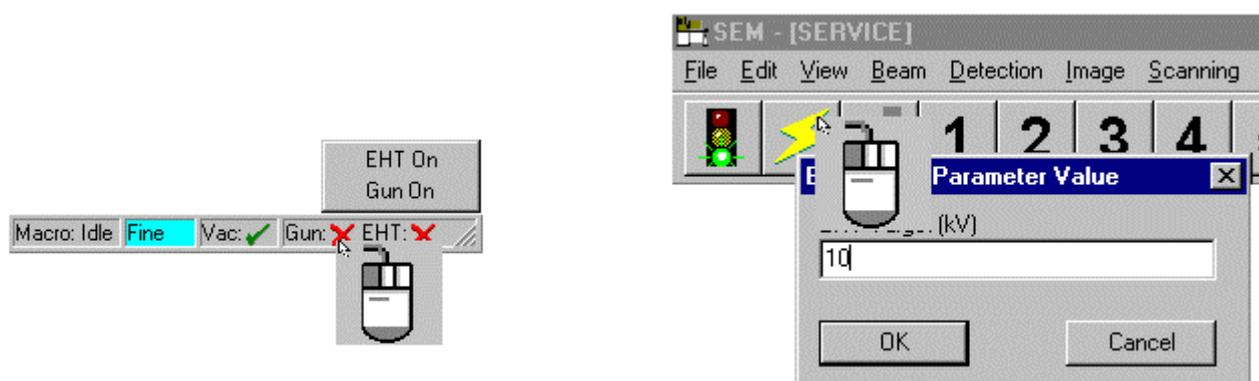
After selection of the corresponding high voltage open the SEM control window (**CTRL+G**) or **TOOLS** → **GO TO CONTROL PANEL**). The index tab **Detectors** (see 4.3.1) enables the selection of a detector. For working distances beyond 10mm select the SE2 detector for the signal source. It is recommended that inexperienced persons have the signal set automatically at the beginning of their work by setting **Signal Adjust** to **Auto BC= BC** (see 4.3.1).
