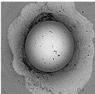
Imaging with a BSE detector. The image shows only small surface contrast, but differences in material can be distinguished very clearly. The topography is imaged weakly.
