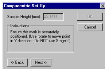
A higher magnification (500X) will automatically be set on the microscope to ensure that the point has been centered accurately. Fine adjustment by means of X and R axis is possible.
