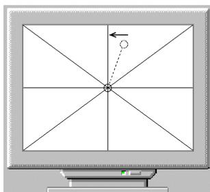
Due to mechanical tolerances, a centered point may drift when tilting from the vertical line. As with the second cycle (8° tilt) this drift can be compensated by means of the function *Compu. Tilt Error*.
