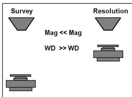
Before switching between the two modes, the settings for the working modes **Survey Mode** (high working distance, small magnification) and **Resolution Image** (small working distance, high magnification) will have to be set.
