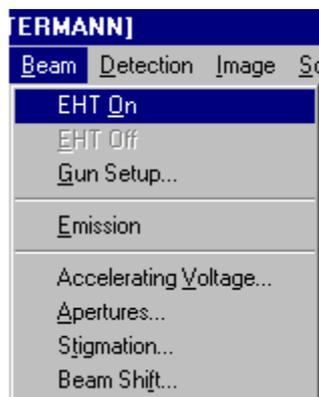
The menu “**Beam**” contains commands and settings important for the adjustment of the electronic beam.
