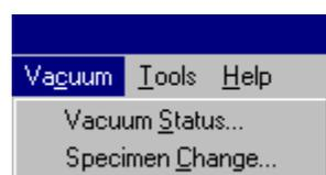
The commands **Vacuum Status...** and **Specimen Change...** will open the **SEM Control-** window, index tab **Vacuum** which contains the most important parameters of the vacuum system. This menu also enables the venting of the sample chamber and the start of the pumping procedure. More detailed information (see 4.3.3.)
