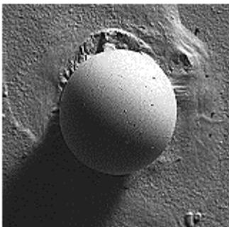
Imaging with the SE2 detector at negative collector voltage (-250V). Only high energetic back-scattering electrons are detected. The image shows an extremely strong topography with shadows. The material contrast is almost completely absent.
