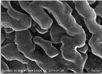
The coating enhances surface structure of chitin, here forming semicrystalline fibrils.
