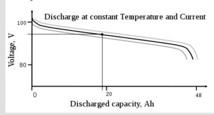
The model shall incorporate Voltage and the instantaneous Current drain as well as the battery Temperature and Internal Resistance/Ageing
