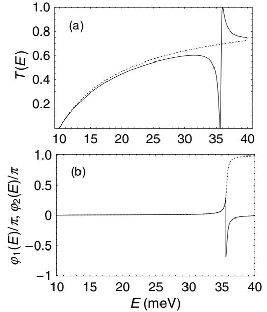
**Figure 7.** (a) Fano resonance in the transmission for a quantum waveguide with a short-range attractive potential (solid line) and a background transmission (dotted line). (b) The phase shift of the amplitude for the electron wave in the first propagating channel (solid line) and the second evanescent channel (dotted line).
