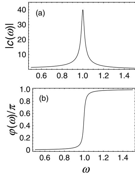
**Figure 1.** (a) The resonant behaviour of the amplitude in the single, driven oscillator as a function of the frequency; where the frequency of the oscillator is in units of the natural frequency,  $\omega_0$ . (b) The phase jump by  $\pi$  near the resonance is shown. (Here, a frictional parameter  $\gamma = 0.025$  is used, and the amplitude is in units of  $a/\omega_0^2$ ).
