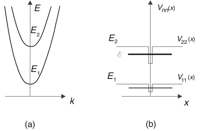
**Figure 5.** (a) Energy dispersion relation for an electron in a perfect waveguide and (b) the diagrams for a bound level (near the first sub-band) and quasi-bound level (near the second sub-band) in the dot's effective potential.
