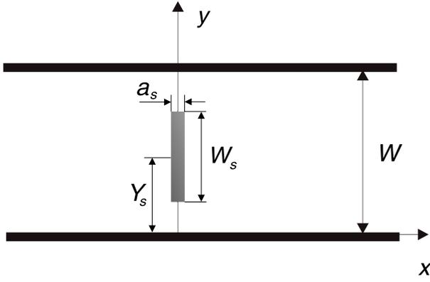
**Figure 4.** Schematic illustration of the electron waveguide with an embedded quantum dot (grey-coloured area); where the attractive potential well is centred at  $x = 0$  and  $y = Y_s$  and the electron motion is not limited horizontally,  $-\infty < x < \infty$ , but is confined vertically,  $0 < y < W$ .
