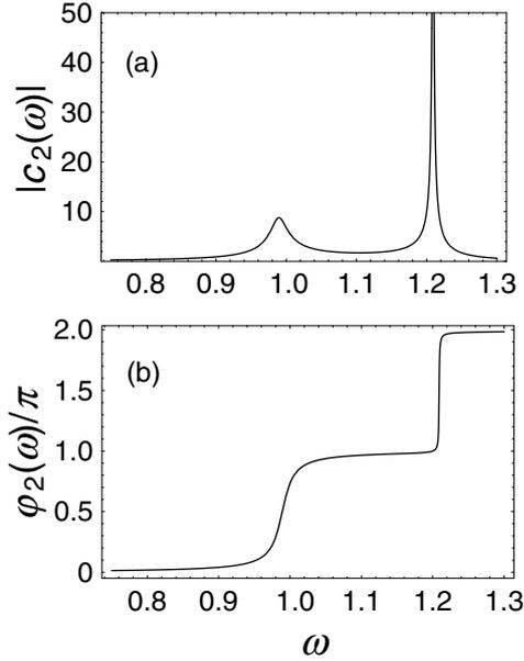
**Figure 3.** (a) The amplitude of the second oscillator as a function of the frequency; where the frequency is in units of  $\omega_1$ . Two symmetric, resonant peaks appear at the eigenmodes of the coupled oscillators. (The modulus of amplitude is in units of  $a/\omega_0^2$ .) (b) The phase behaviour of the second oscillator; where a sequential phase change by  $\pi$  is seen as the driving frequency passes through the resonances.
