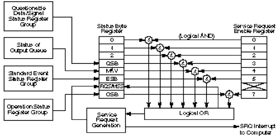
**Figure 3-7. Status Byte and Service Request Enable**
