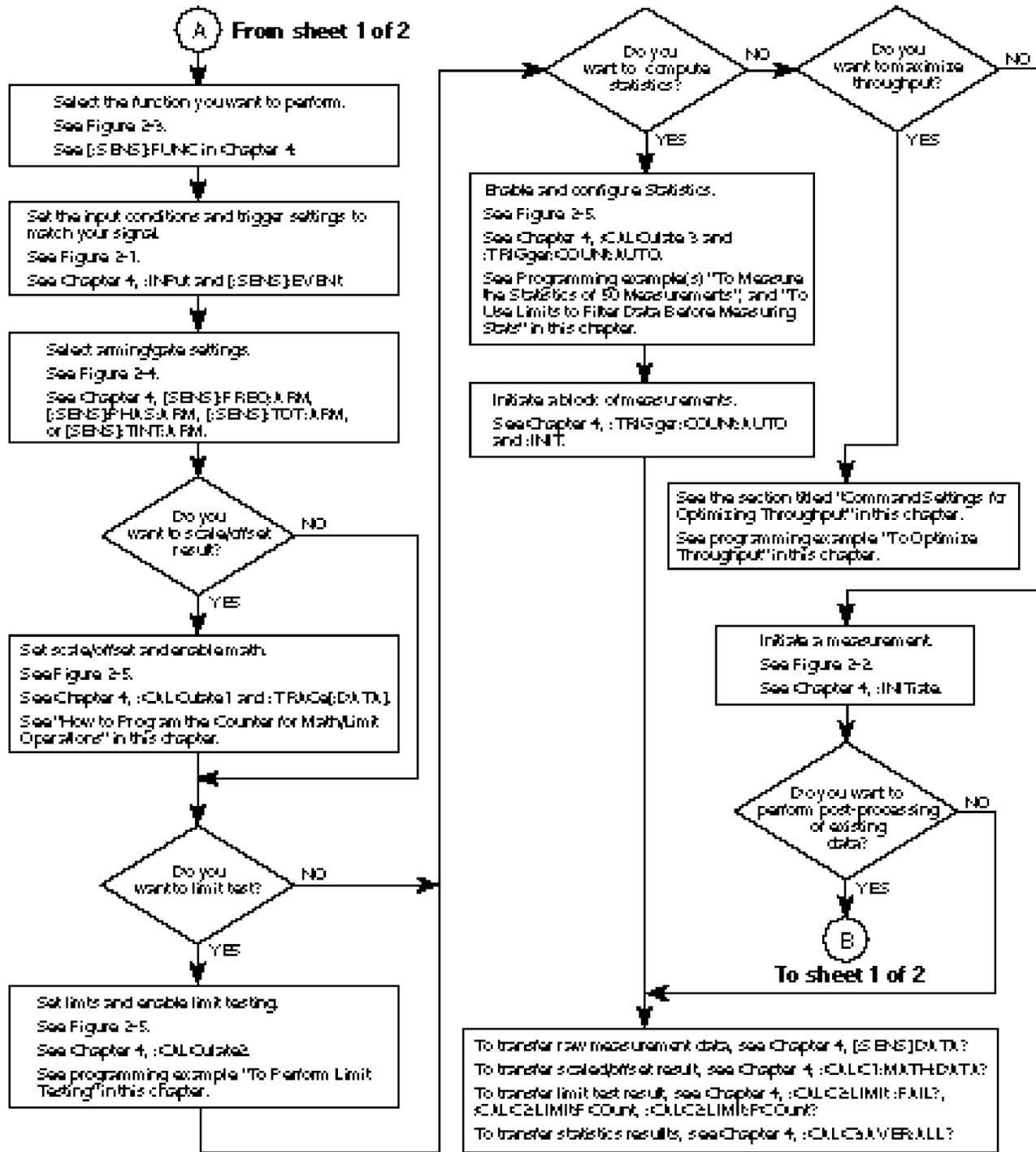
Figure 3-11. SCPI Programming Flowchart (Sheet 2 of 2)
