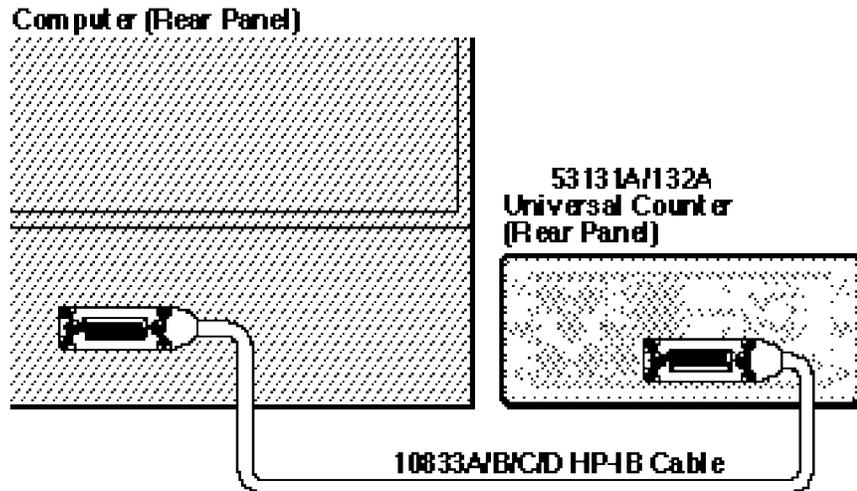
**Figure 3-1. GPIB Interconnection**
