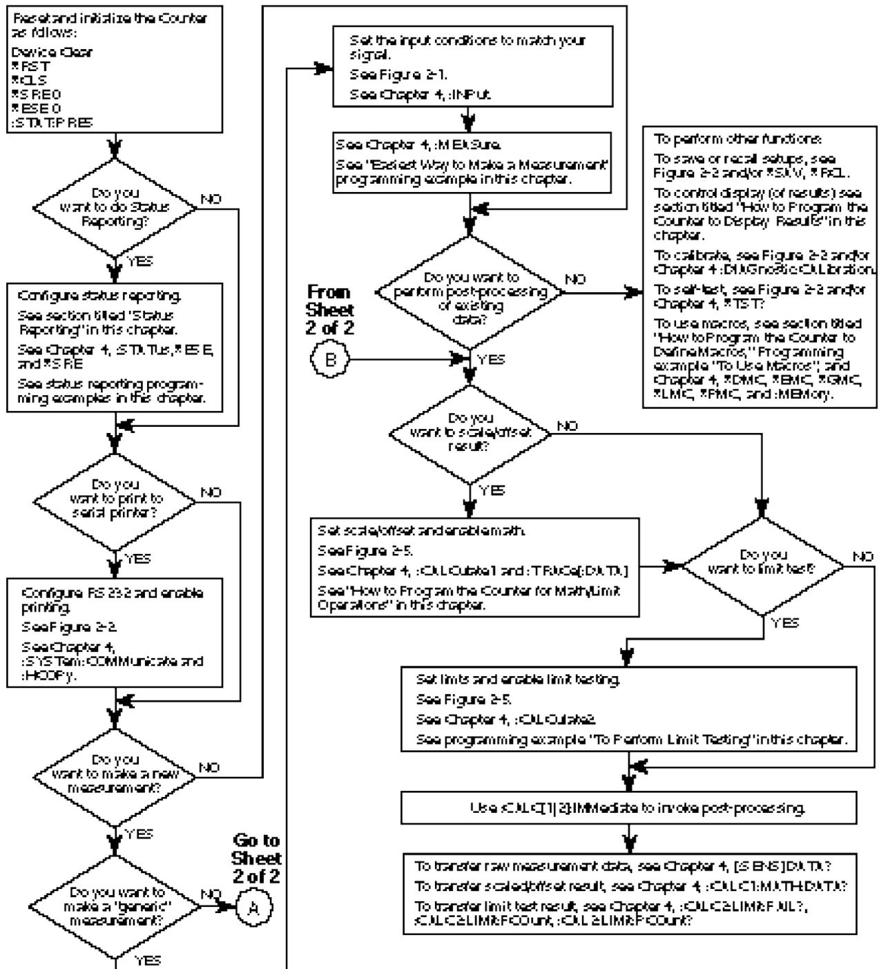
Figure 3-11. SCPI Programming Flowchart (Sheet 1 of 2)
