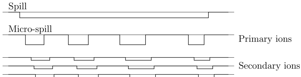
Figure E.1: The micro-spill structure can theoretically be shifted for different isotopes due to their velocity dispersion.
