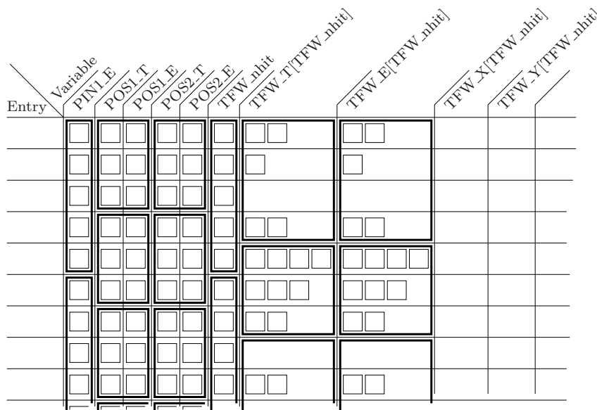
Figure 5.2: HBOOK column-wise ntuple files and ROOT trees are stored with individual variables or groups in buckets, each containing data from many events. This allows analysis (e.g. plotting) to operate on only a few of the available items per entry while accessing the storage media in large continuous chunks. The figure is not to scale — the number of events in each bucket is much larger in reality.
