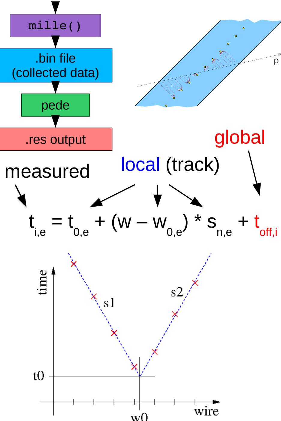
Given data for **many** tracks, pede solves for the **global** parameters, as if all tracks with **all local** and **global** parameters are fitted *simultaneously*
