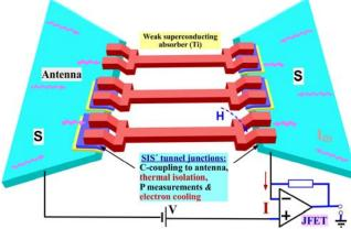
For combination of effective HF operation and low noise properties, the current-biased SCEBs are connected in parallel for HF signal and in series for DC. A signal is concentrated from an antenna to the absorber through the capacitance of the tunnel junctions and through additional capacitance for coupling of superconducting islands.
