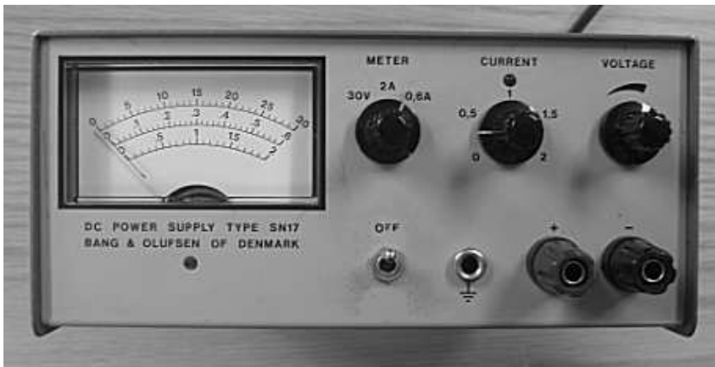
Figur 14: Likspänningsaggregat BoO SN17
