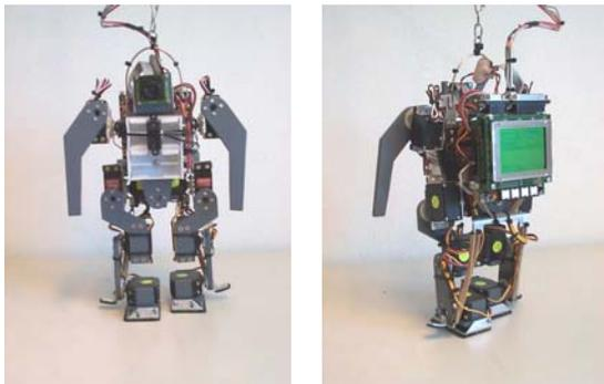
**Figure 4.** Pictures of the ELVINA Humanoid. Camera and PSD sensor visible (left) and controller board (right).
