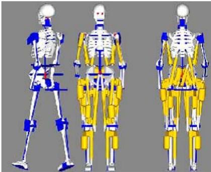
**Figure 2.** CAD-drawings of Priscilla showing skeleton, titanium reinforcements and actuators.
