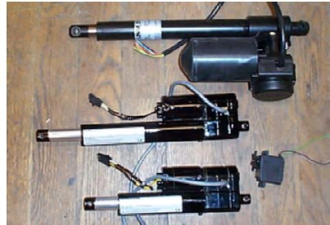
**Figure 3.** Picture of the actuators and servo. From top to bottom La30, La1 with stroke 0.115m and 0.06m respectively. To the right the R/C-servo.
