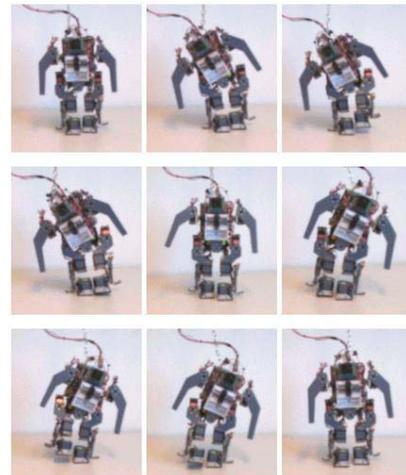
**Figure 5.** Series of pictures showing a complete gait cycle, from top left to bottom right.
