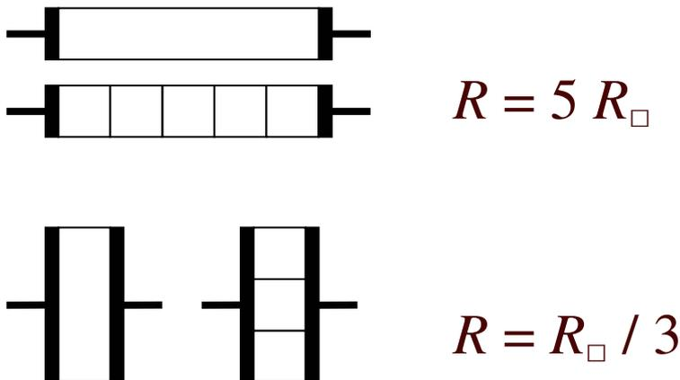
Figure 3. To get the actual resistance of a strip, just count up the number of squares which fit inside the strip. Black bars represent equipotential contact pads with resistances negligibly smaller compared to the resistance of thin film.
