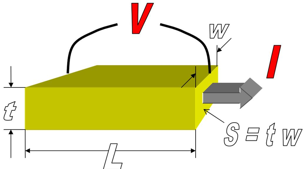
Figure 1. Elementary geometry of resistance measurements.
