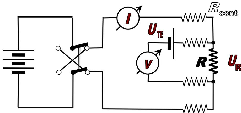
Figure 11. Bias reversal schematic.
