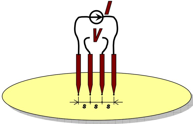
Figure 10. Sheet resistance of a large-area thin film.
