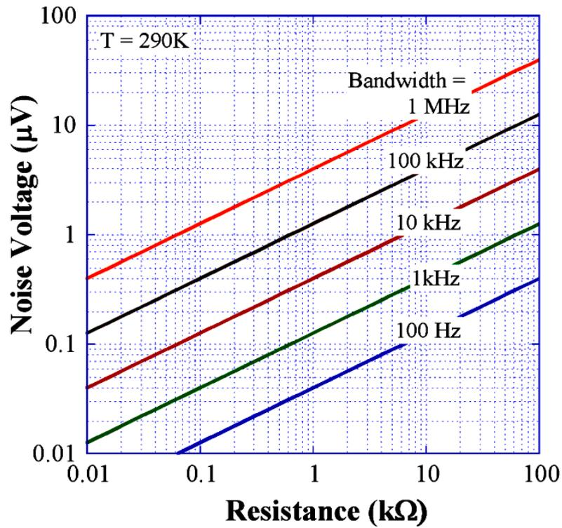
Figure 13. Thermal noise voltage as a function of resistance and bandwidth
