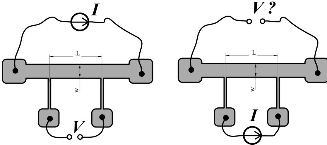
Figure 6. Thin film of thickness  $t$  patterned into a slab of width  $w$ . The distance between the voltage contacts is  $L$ .
