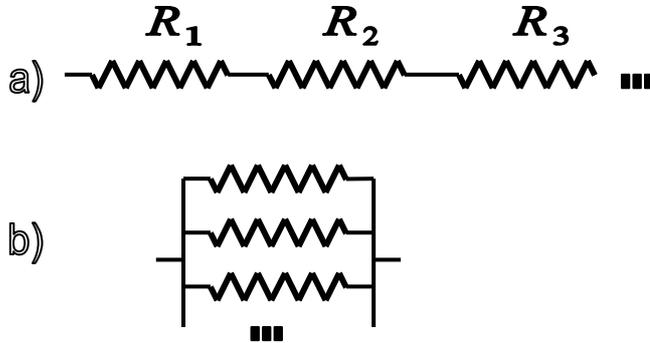
Figure 2. Resistances connected in series (a) and in parallel (b). For  $N$  serially connected resistors,  $R = R_1 + R_2 + R_3 + \dots + R_i + \dots + R_N$ . For  $N$  resistors connected in parallel,  $1/R = 1/R_1 + 1/R_2 + 1/R_3 + \dots + 1/R_i + \dots + 1/R_N$ .
