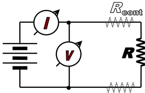
Figure 4. Two-probe resistance measurements. Unknown contact resistance gives error.
