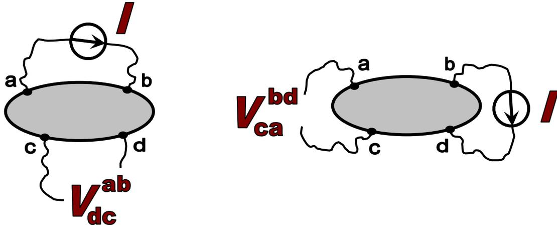
Figure 8. Van der Pauw method of resistivity measurements of a thin film of arbitrary shape.
