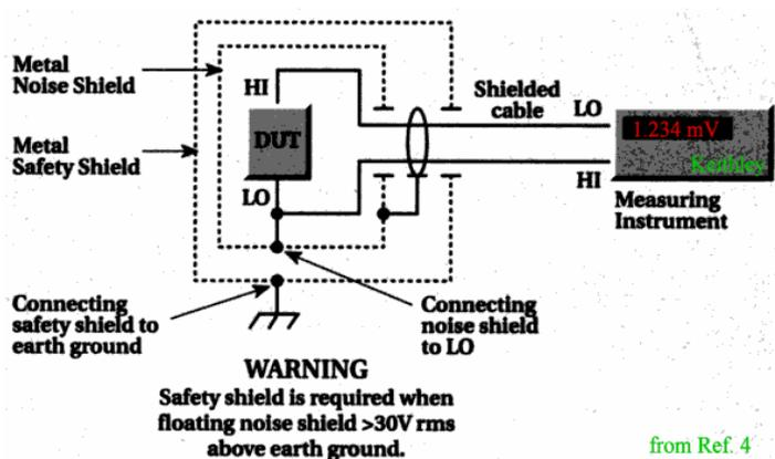
Figure 12. Shielding from RFI/EMI signals (from Ref.4)
