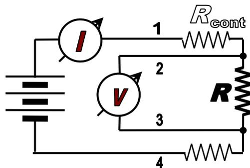
Figure 5. Four-probe resistance measurements. Contact resistance does not contribute to the voltage  $V$ . Probes 1 and 4 are usually called “current probes”, while 2 and 3 – “voltage probes”.
