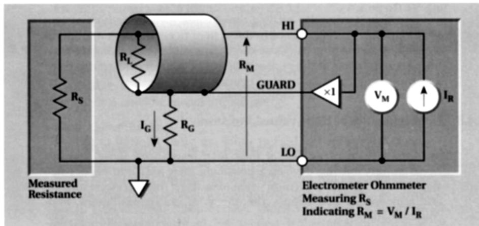
Figure 14. Guarding cable shield to eliminate leakage resistance. (from Ref. 1&4)
