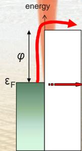
$$\phi = \phi_0 - \alpha T - \sqrt{\frac{eE}{4\pi\epsilon_0}} \quad \Delta\phi_{[eV]} \sim 3.8 \times 10^{-5} \sqrt{E_{[V/m]}}$$
