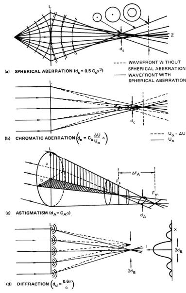
FIGURE 2.28. Aberrations and diffraction. (a) Spherical aberration ( $d_s = 0.5 C_s \alpha^3$ ) (---, wavefront without spherical aberration; —, wavefront with spherical aberration); (b) chromatic aberration [ $d_c = C_c (\Delta U / U_0) \alpha$ ] (---,  $U_0 - \Delta U$ ; —,  $U_0$ ); (c) astigmatism ( $d_A = C_A \alpha$ ); (d) diffraction ( $d_d = 0.6 \lambda / \alpha$ ).
