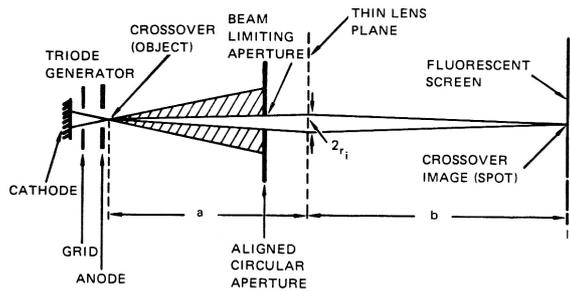
FIGURE 2.24. Gun configuration for beam fabrication.
