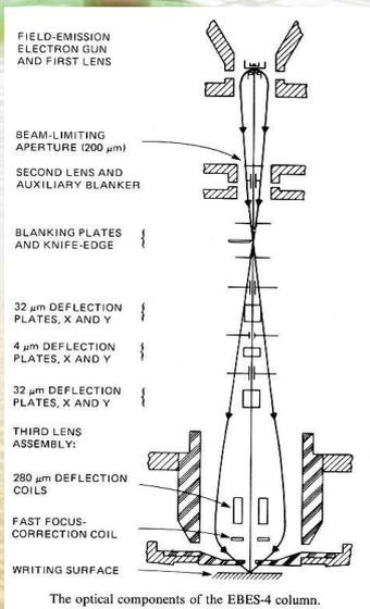
The optical components of the EBES-4 column.
