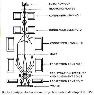
Reduction-type electron-beam projection system developed at IBM.
