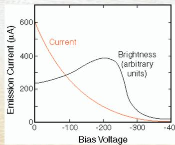
A bias resistor allows the gun to be self-regulating. Any increase of the emission current causes a larger voltage drop across the bias resistor and a larger negative voltage is applied to the Wehnelt, reducing the current. As the emission increases, so does the voltage difference between Wehnelt and filament, causing the emission to saturate. Proper bias voltage also optimizes the electron beam brightness.
