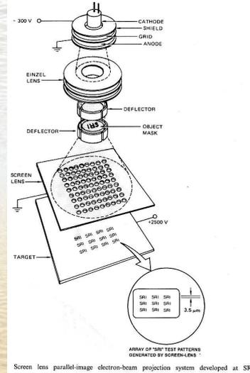
Screen lens parallel-image electron-beam projection system developed at SRI
