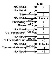
Figure 4-3. The Questionable Data/Signal Status Register Group
