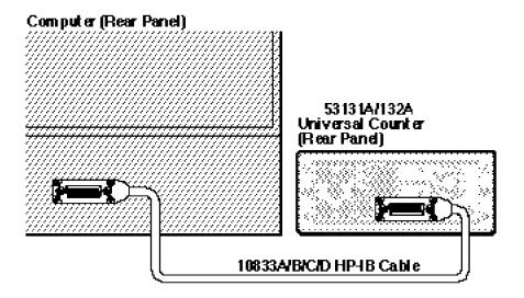
Figure 3-1. GPIB Interconnection
