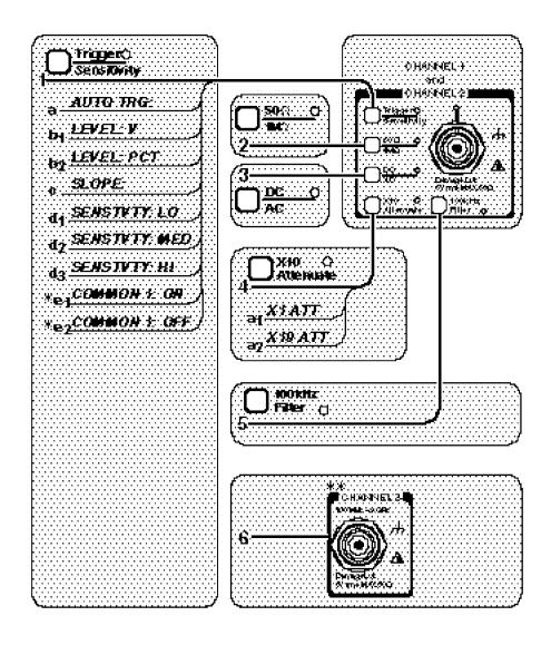
Figure 2-1. Input Channels Conditioning Keys to SCPI Command Map (Part 1 of 2)
