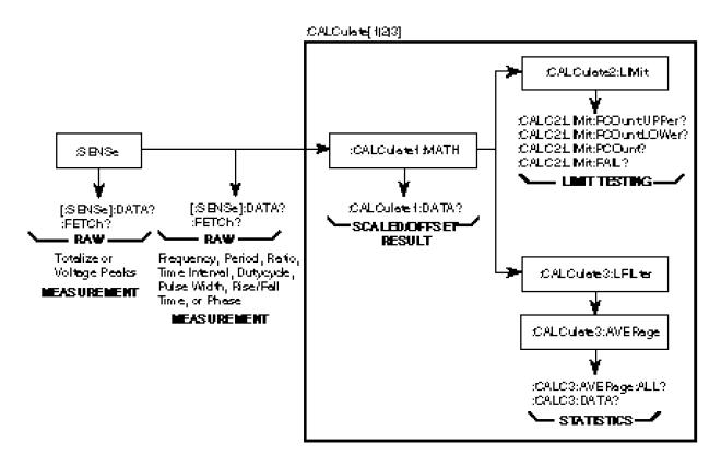
Figure 4-1. The CALCulate Subsystems
