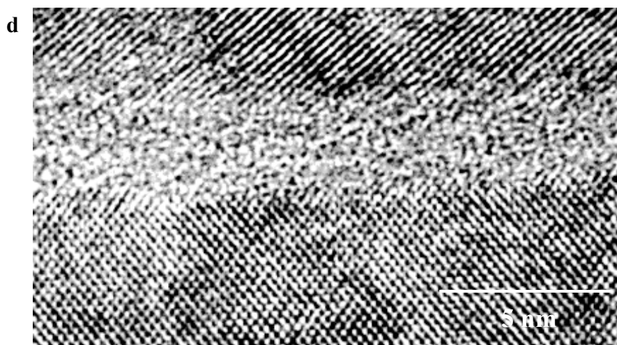
Figure 1: High resolution cross-sectional TEM of Si/SiO 2 /poly-Si 1-x Ge x . (a) sample S1, (b) sample S2, (c) sample S3 and (d) sample S4.
