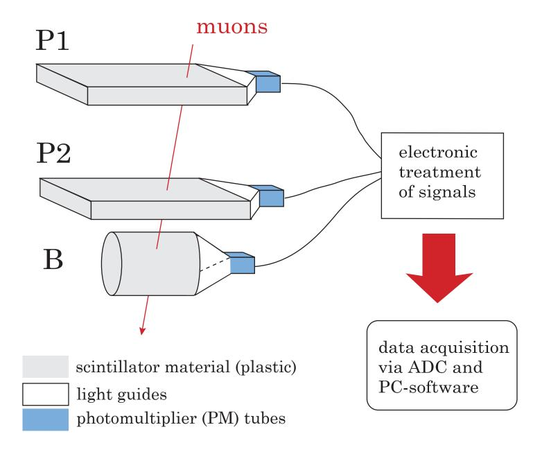
P1 : Paddle 1 (in the roof)P2 : Paddle 2 (just above B)B : Barrel (lying on the floor)
