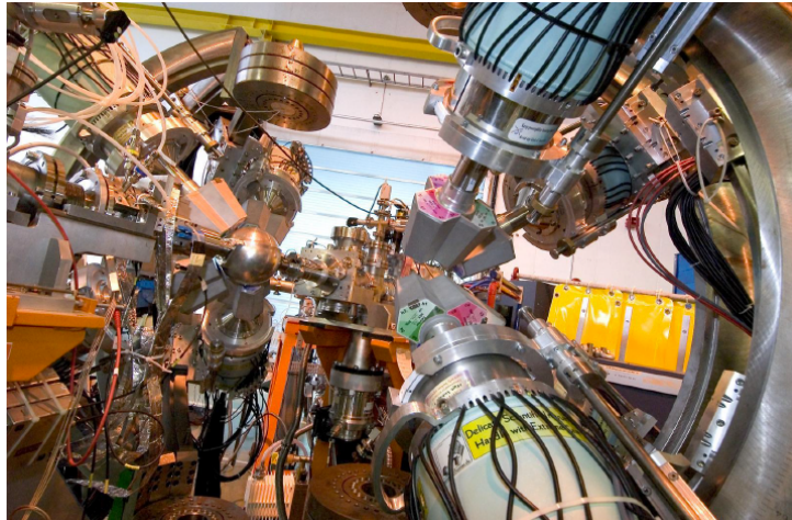
Fig. 7. The Miniball germanium detector array, developed for low-intensity RIB experiments, is shown in its retracted position. The germanium detectors surround a set of segmented silicon detectors that are placed in closed geometry in the spherical reaction chamber.
