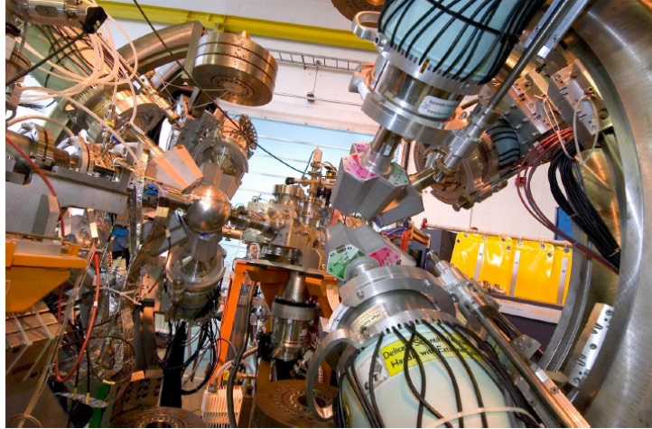
Fig. 7. The Miniball germanium detector array, developed for low-intensity RIB experiments. The germanium detectors surround a set of segmented silicon detectors that are placed in closed geometry in the spherical reaction chamber.
