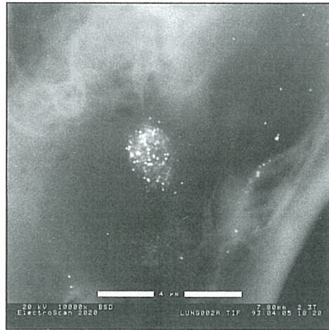
Figure 5-19, Left - Lung tissue labeled with 20 nanometer gold particles. A gold coating would have obscured the labeling particles
