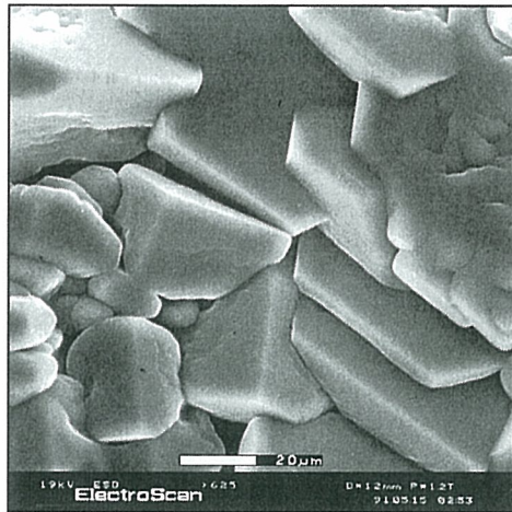
Figure 5-22, Left - Ice crystallized from vapor in the ESEM
