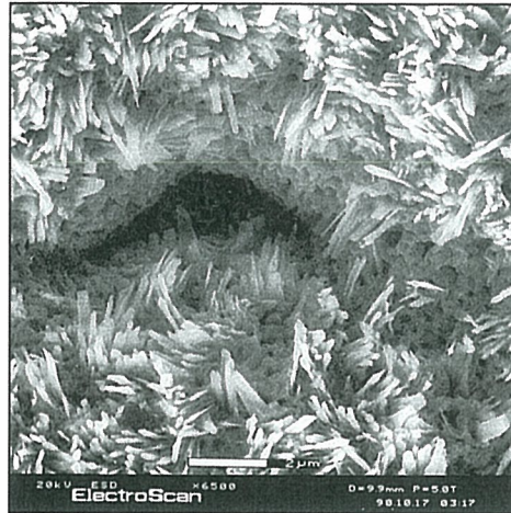
Figure 5-24, Left - Oxide grows around a small sulfur inclusion in a piece of iron at 860°C in a pure oxygen atmosphere Right - Iron sulfide crystals grown on stainless steel
