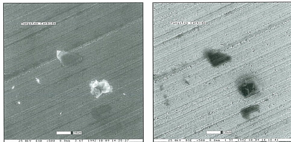
Figure 2-8. This sample shows light element particles on a tungsten carbide substrate. The SE image (left) shows mostly topographic contrast. Note the surface detail of the particles. Contrast in the BSE image (right) is due primarily to differences in atomic number.
