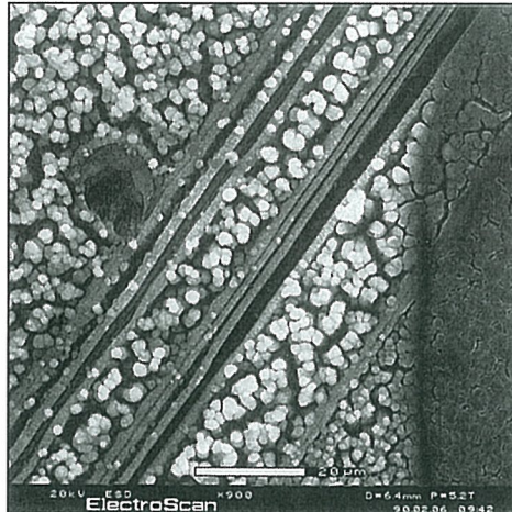
Figure 5-25, Left - A droplet of liquid toluene has etched away the matrix of a plastic composite Right - In a high temperature oxidizing environment, cracks develop at the fiber/matrix interface of a silicon carbide reinforced composite.
