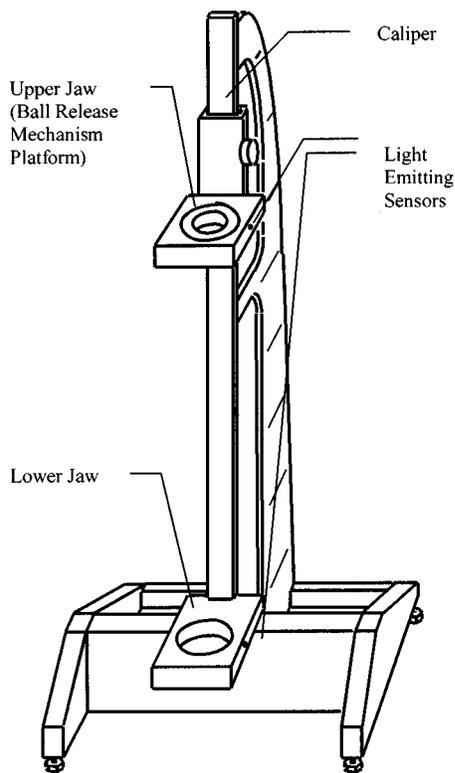
Fig. 1. The apparatus (the release mechanism is not shown).
