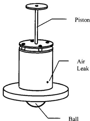
Fig. 2. The ball release mechanism.
