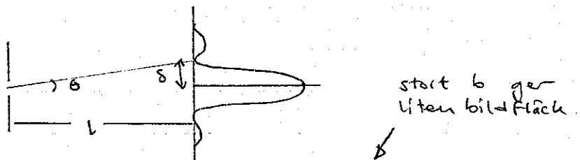
$$\begin{aligned} 1:a \text{ min: } b \cdot \sin \theta &= \lambda \\ \sin \theta \approx \frac{\delta}{l} \end{aligned} \quad \Rightarrow \delta = \frac{\lambda}{b} \cdot l$$
