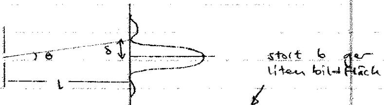
$$\begin{aligned} \text{1:a min: } b \cdot \sin \theta &= \lambda \\ \sin \theta &\approx \frac{s}{l} \end{aligned} \Rightarrow s = \frac{\lambda}{b} \cdot l$$
