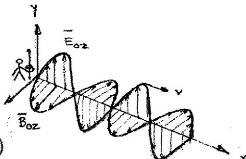
$$\bar{E}_y(x,t) = \bar{E}_{oy} \sin \omega \left( \frac{x}{v} - t \right)$$
