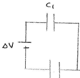
$$\Rightarrow C_s = \frac{C_1 \cdot C_2}{C_1 + C_2} = \frac{25,0 \cdot 5,00}{30,0} \mu\text{F} = C_2$$
