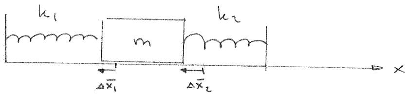
$$\text{Free body diagram: } \boxed{\text{mass}} \rightarrow \widehat{F} = -k_1 \widehat{\Delta x}_1 - k_2 \widehat{\Delta x}_2$$
