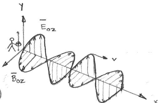
$$\bar{E}_y(x,t) = \bar{E}_{0y} \sin \omega \left( \frac{x}{v} - t \right)$$
