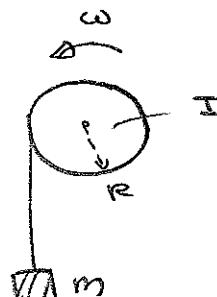
$$\begin{aligned} v &= \omega R \\ \Rightarrow \omega &= \frac{v}{R} \end{aligned}$$
