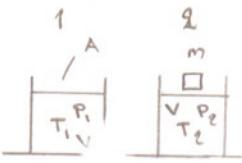
$$\left. \begin{array}{l} P_2 V = n R T_2 \\ P_2 = P_1 + \frac{mg}{A} \end{array} \right\} \Rightarrow \left( P_1 + \frac{mg}{A} \right) V = n R T_2 \quad (2)$$
