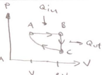
$$T_C V_C^{\gamma-1} = T_A V_A^{\gamma-1} = T_C = T_A \left( \frac{V_A}{V_C} \right)^{\gamma-1}$$
