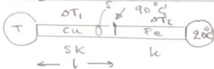
$$\Delta T_1 + \Delta T_2 = T - 20, \quad \Delta T_1 = T - 90$$
